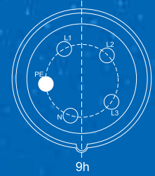
Position of the Earthing Contact
