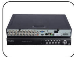
GI-681 16 Channel DVR Full D-1 With Real Time (H.264)
